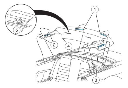
1. Install the boot on the vehicle by hooking the boot retaining clips on the back panel.
